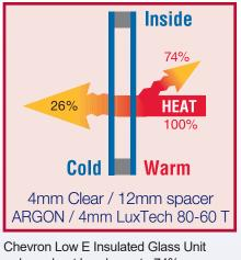
reduces heat loss by up to 74% over single clear glazing
