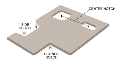
Notches are generally processed by Waterjet Cutter and supplied with flat ground finish with arris.
