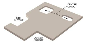
Cut outs are generally processed by Waterjet Cutter and supplied with flat ground finish with arris.
