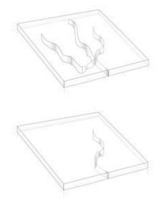
A glass fracture can be identified as a thermal stress breakage if the start of the crack is at 90° to both the edge of the glass AND the face of the glass. Depending on the magnitude of the stresses involved, the crack may only travel for a few millimetres before branching out or veering off-line, so the 90° angle of the initial fracture may not always be immediately apparent.
